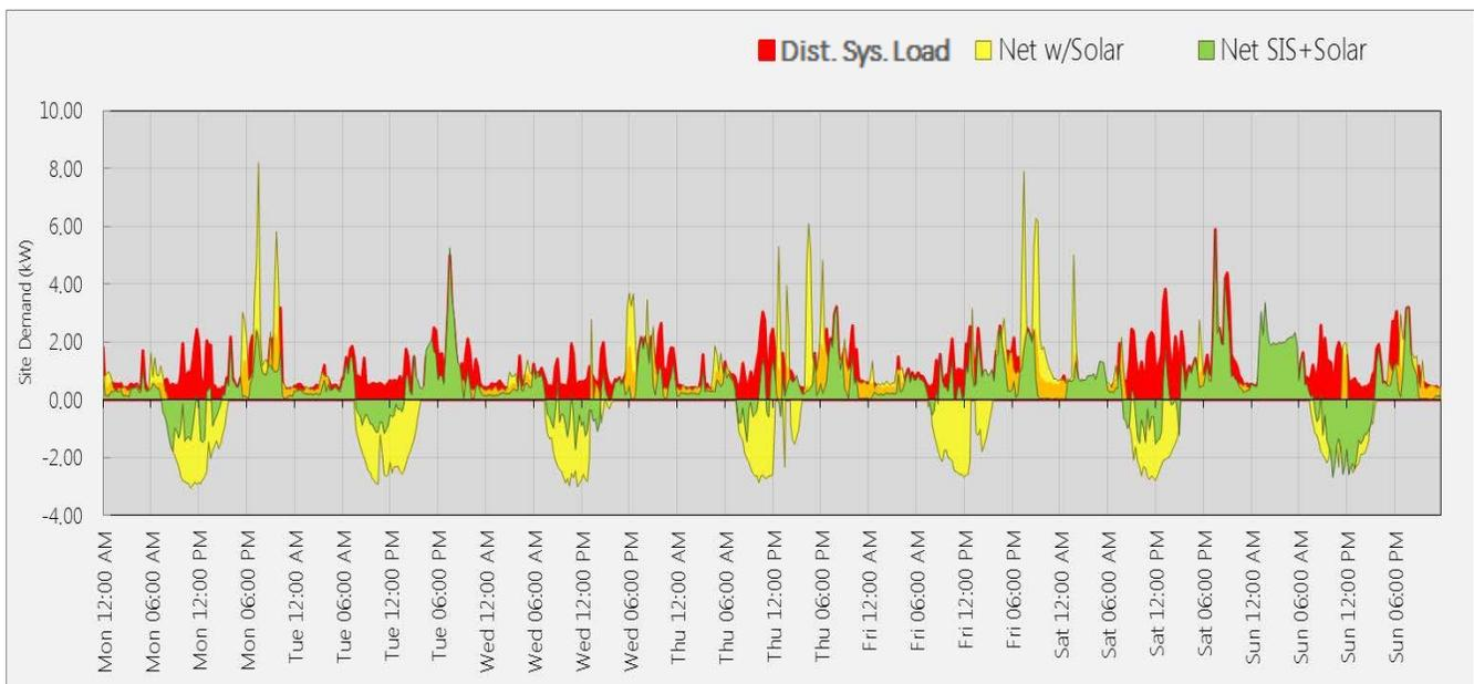
Fig. 6: Compilation of solar and battery impacts on home electricity loads. This graph is an average across the weeks in November.
