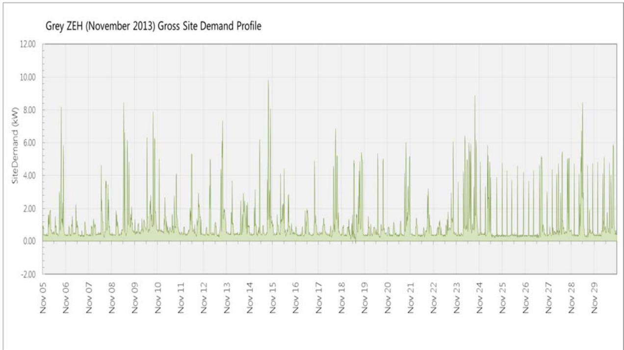
Fig. 5: Electric Load Profile of ZNE Home for most of November 2013. This data is post-ZNE retrofit, and the home is very efficient.
