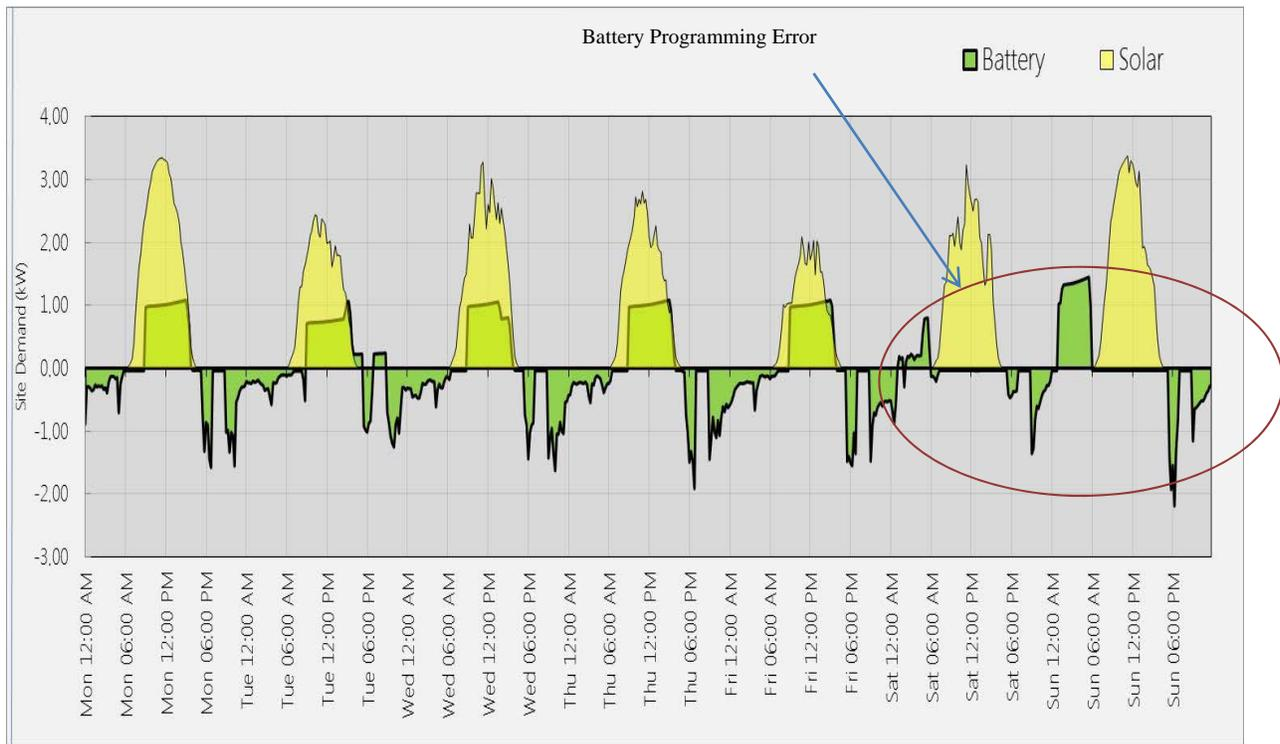
Fig. 4: Solar and battery activity. These data are weekly averages for the solar generation and battery charging and discharging during the month of November 2013. The green shaded area is the battery charging (above zero) or discharging (below zero) to meet home loads.
