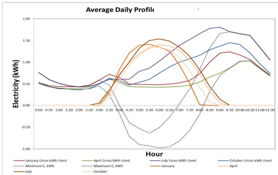
Fig. 1: Simulation results of a BEopt E+ v1.3 model of the CSI RD&D ZNE test home were used to determine the average daily electrical use profile, indicating both gross and net electrical consumption. The average hourly solar generation for the region of California Climate Zone 10 is also shown.
