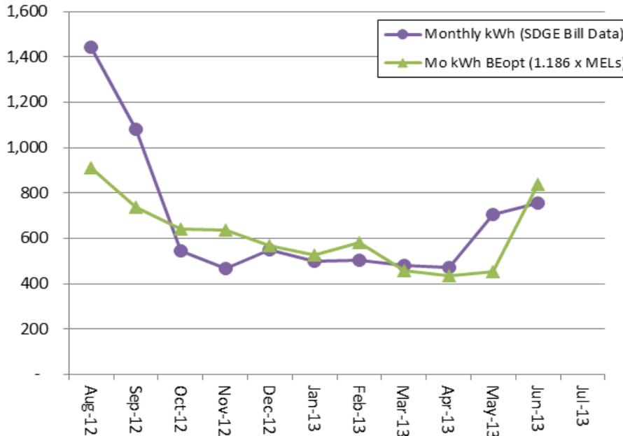
Fig. 2: Baseline data - actual monthly actual energy use from SDG&E bill data and BEopt simulation results for the Santee home. This data is from the 10th of each month labeled in the abscissa to the 10th of the next month (SDG&E meter-reading intervals). The beta-test PV system was installed in Oct 2012, and the generated electricity is accounted for in the SDG&E data.
