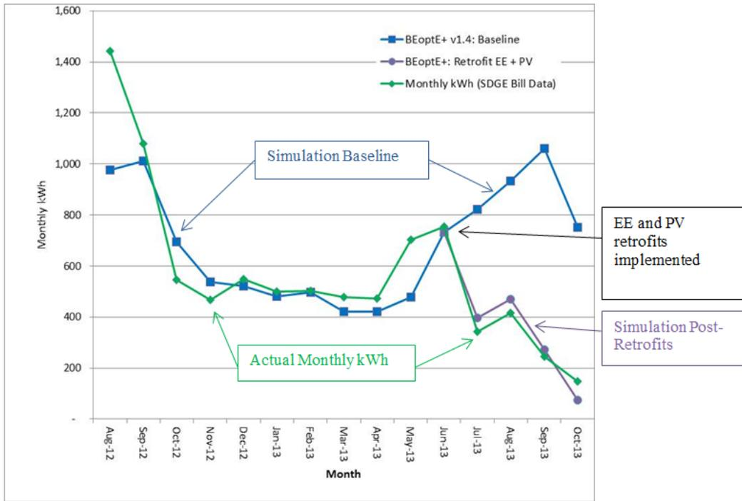
Fig. 3: Baseline and post-retrofit electricity use in ZNE home. Monthly kWh from SDG&E Bills are plotted in green, and BEopt simulation of the baseline electricity use are plotted in blue (pre-retrofit, and the baseline continuing post-retrofit). BEopt simulations of post-retrofit electricity use are plotted in purple, starting the month before the retrofits were performed (June) for continuity in the graph.
